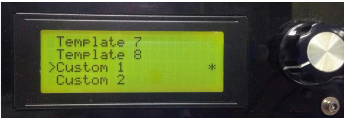
Note: the“\*” after the template means the current template you are choosing and using. System will follow your last chosen operation by default.
