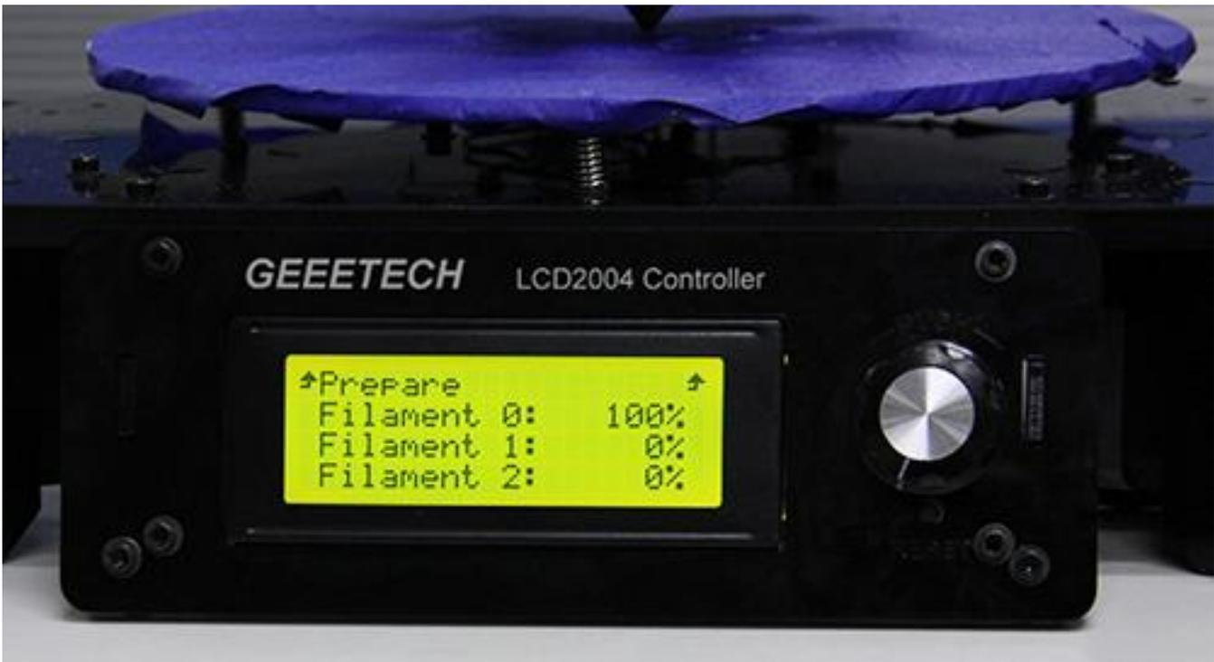
The sum of the proportion of Filament 0, Filament 1 and Filament 2 is 100%. If you manually adjust either of the two values, system will automatically work out the other value. The proportion will not change unless you readjusting it or choosing template again.
