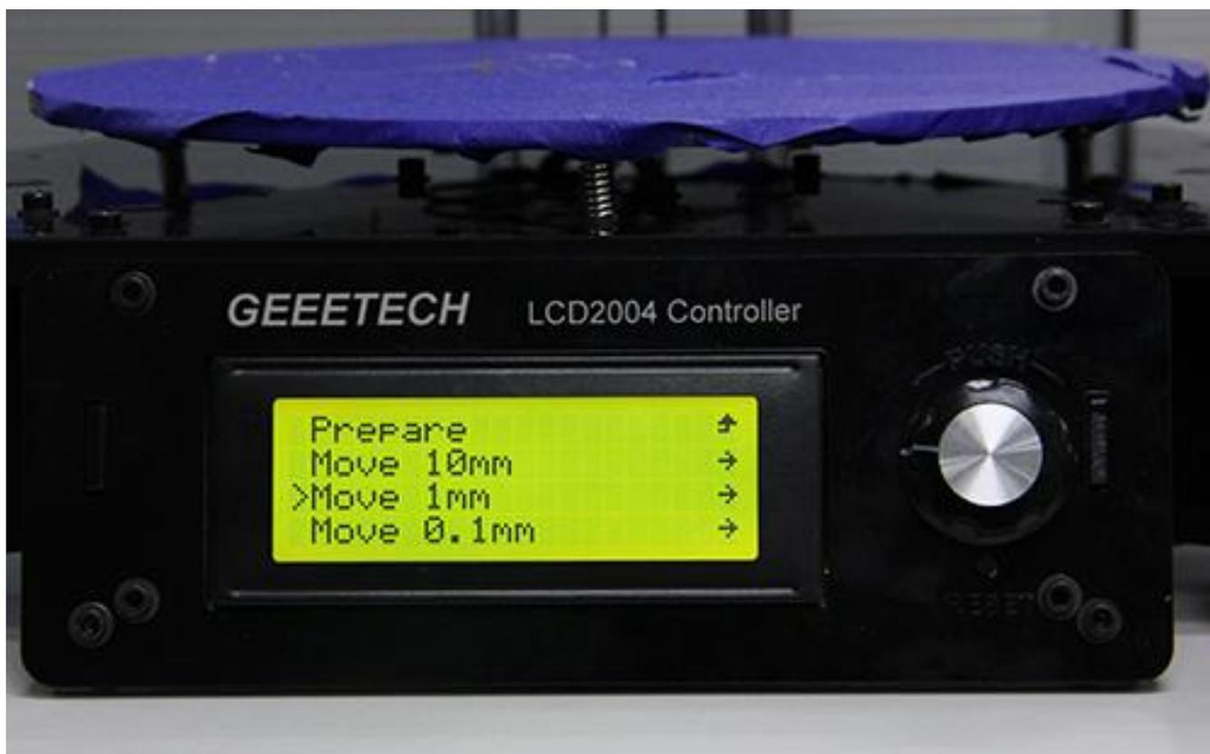
Choose the axis you need to move: Move **X/Y/Z** to test the 3 axis. Move **E0/E1/E2** to test the extruder. Rotating the knob can make each axis move.
